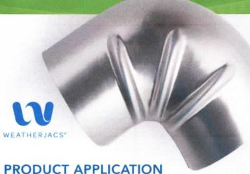
In accordance with ASTM 1729, WeatherJacs® are 2-piece pressed fittings which are pre-formed for 45 & 90 degree insulated bends conforming to ASTM, C-585 & C-450 standards. Available sizes range from ½" up through 30" NPS in long and short radius. Socket weld sizes are available from ½" through 3".
